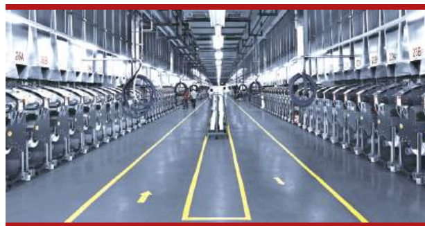
The WINGS family from Oerlikon Barmag covers almost every process; standard, high-titer or micro yarns, polyester or polyamide, POY or HOY, 10-, 12-, 20- or even 24-thread.
